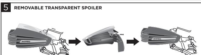
**Remove the spoiler by removing the internal screw.**
